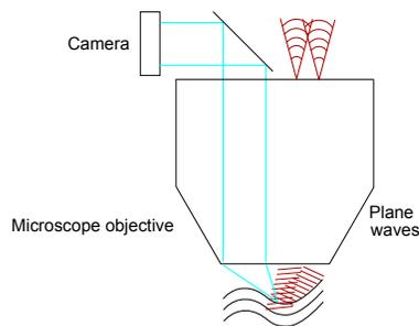
Fig. 11. Setup for single-shot topographic measurements
