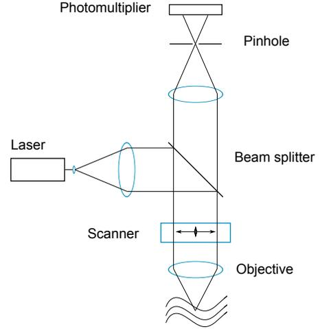
Fig. 1. Schematic setup of a confocal microscope
