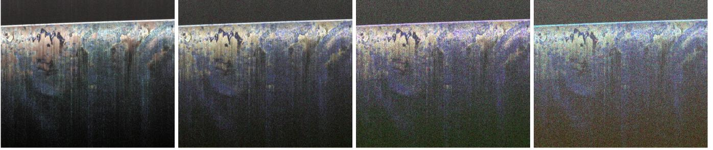
DOCT contrast calculated with different sized sequences (left to right) on a trachea (top), ovar (middle), and colon (bottom) sample. One can see that even just 4 frames can provide a sufficient dOCT image to distinguish different tissues by activity, even though the images are noticeably noisier.
