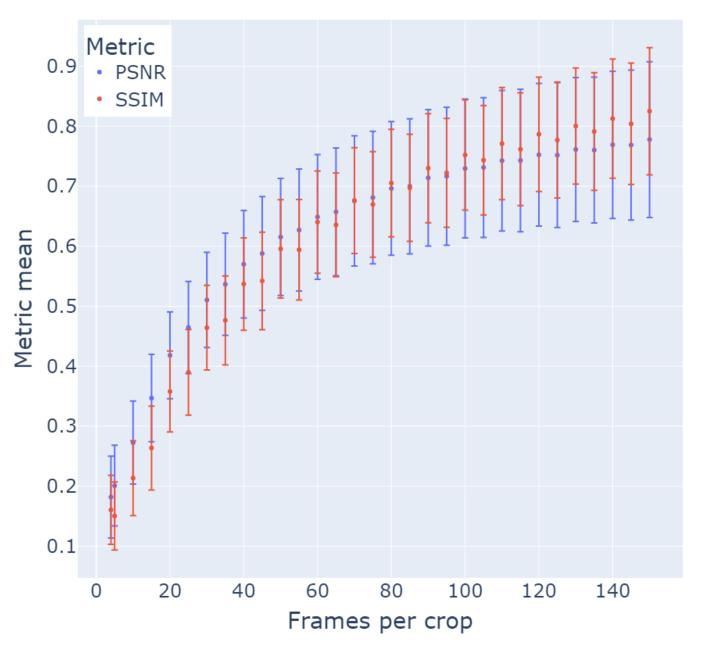
Peak-Signal-to-Noise-Ratio (PSNR) and Structural-Similarity (SSIM) over frames per crop. Both decrease in a similar way for shorter time series, indicating the nonlinear increase of spectral noise.
