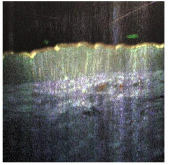
Pixelwise Fourier Transformation over the B-Scan time series yields a frequency spectrum of the signal changes for each pixel. Binning these into 3 channels results in an RGB image.
