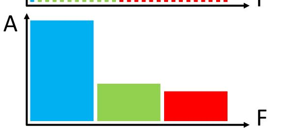
Schematic illustration of how a real spectrum (top) may look like depending on the sampling and how it would be binned (middle and bottom). Fewer frames decrease the spectral resolution.
