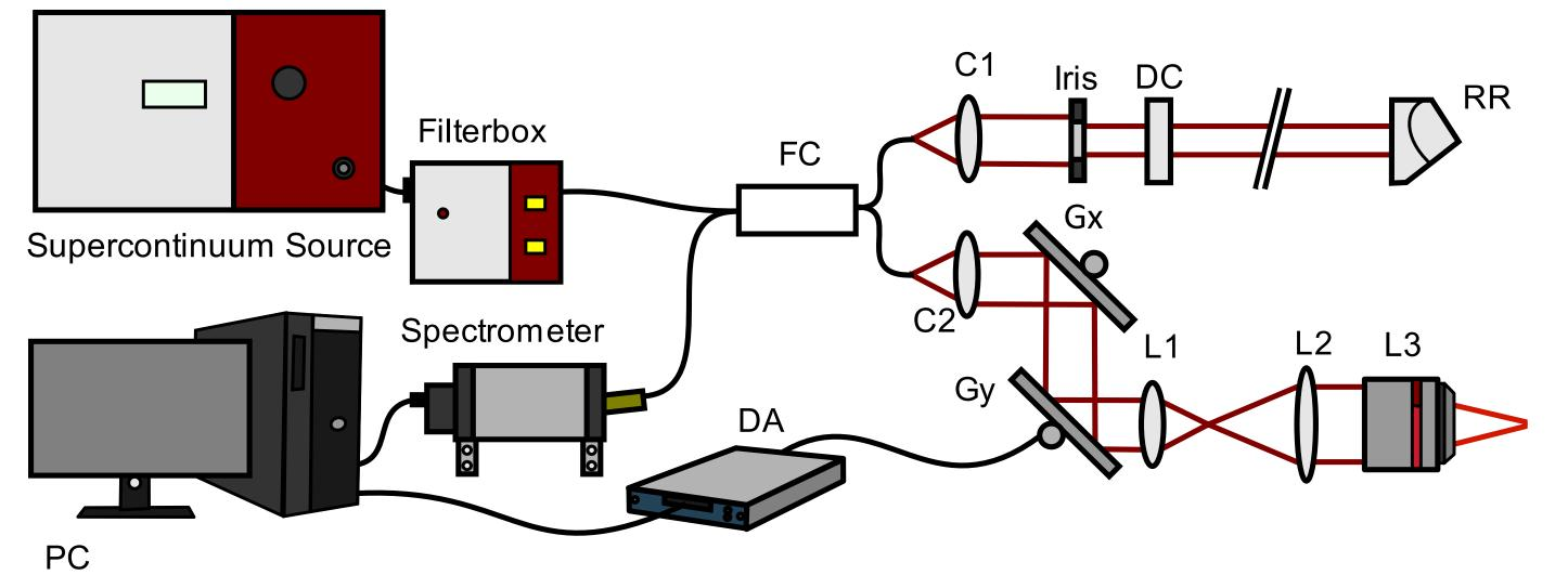
Our custom build OCT setup with microscopical resolution. FC: Fiber-coupler, C: Collimator, DC: Dispersion Correction, RR: Reference Reflector, G: Gyroscopic mirror, L: Lens, DA: Digital-Analog-converter
