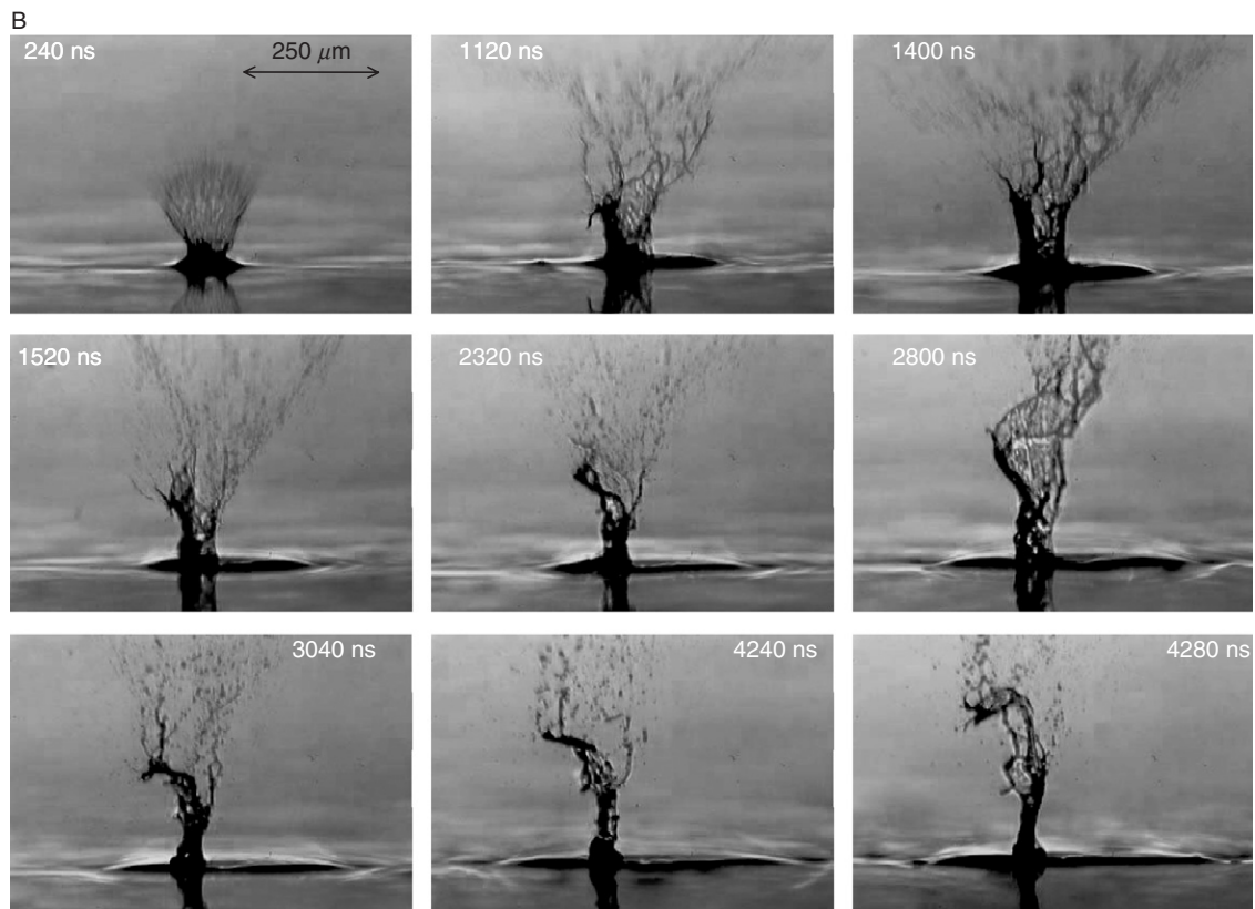
Fig. 24 Catapulting of cell preparations (CHO cells on PEN foil) out of a duplex dish. The liquid layer between Teflon membranes and PEN foil was 30- to 50- \mu\text{m} thick, and a 10- to 50- \mu\text{m} -thick layer of culture medium covered the cells. (A) Catapulting with defocused laser pulses and (B) catapulting with pulses focused at the periphery of the specimen (the plasma luminescence indicates the location of the laser focus). 20 \times objective, NA = 0.5, E = 20 \mu\text{J} , and specimen diameter 100 \mu\text{m} . The average specimen velocity during the first 4 \mu\text{s} is about 50 m/s in (A) and 55 m/s in (B). The rotational movement of the specimen in (B) corresponds to a frequency of 220,000 rps during the first microsecond and 125,000 rps when averaged over the first 4 \mu\text{s} .
