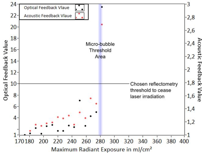
Figure 2 Quantification of micro-bubble induced characteristics of the optical and acoustical signals over the applied maximum radiant exposure.
