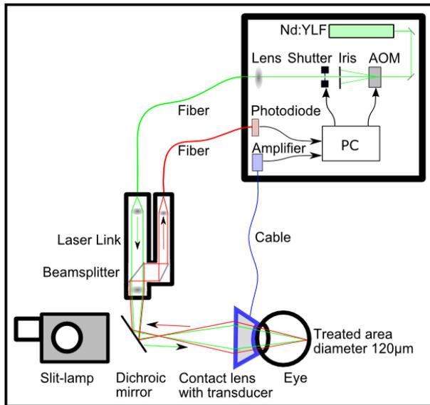
Figure 1 The Setup: A PC-system controls the laser irradiation by an AOM and a shutter. An optical system (laser link) projects a spot of desired size to the retina. Backscattered light is guided to a photodiode. Acoustic transients are acquired by an ultrasonic transducer. The optical and acoustical signals were analyzed for micro-bubble induced characteristics. The laser irradiation is ceased automatically upon bubble formation.
