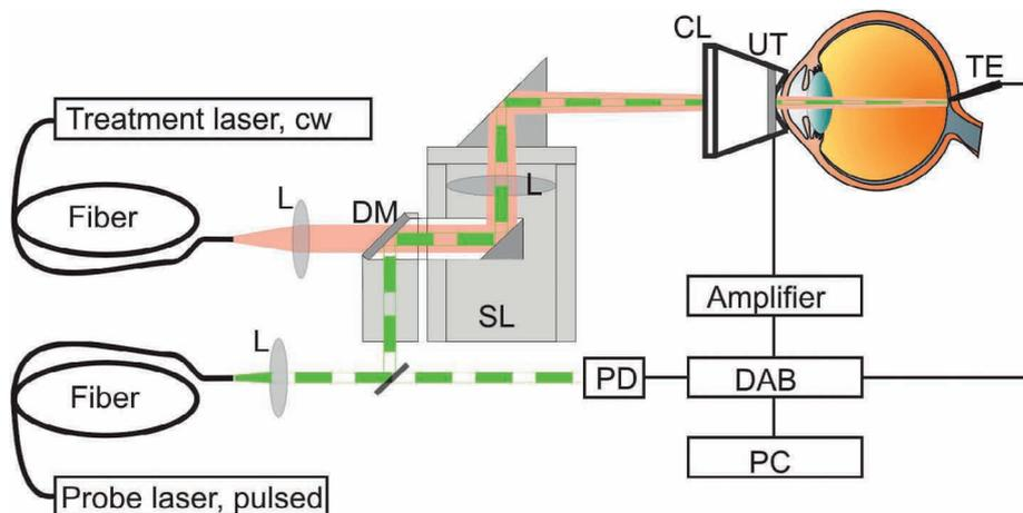
**Figure 2:** Experimental setup for optoacoustic temperature determination during cw-laser irradiation. L: lens, DM: dichroic mirror, SL: slit lamp, PD: photo diode, CL: contact lens, UT: ultrasonic transducer, TE: thermo couple (ex-vivo only)
