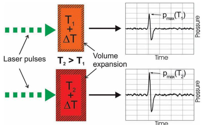
Figure 1: Principle of optoacoustic temperature determination
