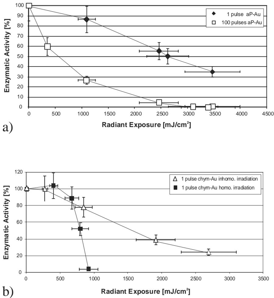
Figure 3: Enzyme activity after irradiation with nanosecond pulses of different radiant exposure.
