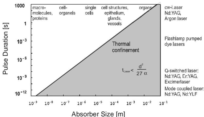
Figure 1: Pulse duration versus absorber diameter for achieving selective thermal effects.
