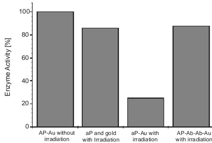
Figure 5: Inactivation experiment irradiating directly and antibody coupled alkaline phosphatase with  $10^4$  pulses of  $54 \text{ mJ/cm}^2$ .
