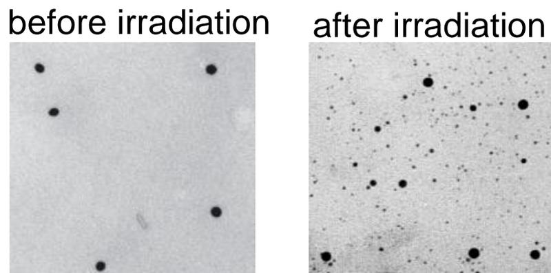
Figure 6: Electron microscopy image of alkaline phosphatase conjugates before and after irradiation with  $10^4$  pulses at  $69 \text{ mJ/cm}^2$ .
