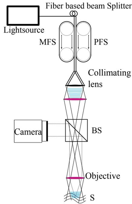
Fig. 5. Schematic setup with fiber based structured illumination and piezo fiber stretcher (PFS), manual fiber stretcher (MFS), a Beamsplitter (BS) is used to guide the reflected light to the camera
