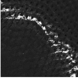
Fig. 3. Image of the wing of a fly with a conventional SIM setup
