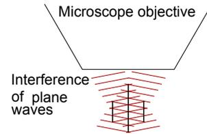
Fig. 2. Schematic illustration of the interference of two plane waves; black points represent lines of constructive interference
