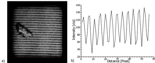
Fig. 6. a) Focused silver mirror with Zeiss 40x/0.75/ $\infty$ /0 WN-Achroplan objective, size:  $145 \times 145 \mu\text{m}$ ; b) plot of intensity profile
