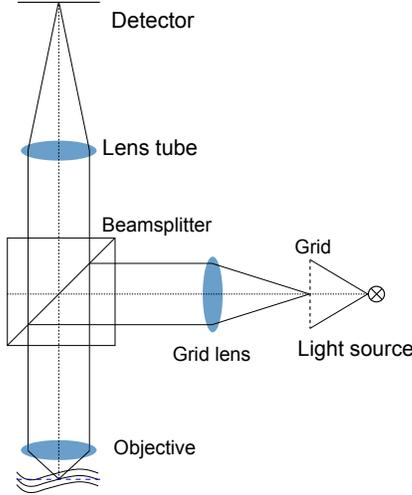
Fig. 4. Conventional SIM-setup
