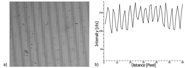
Fig. 7. a) With conventional SIM focused silver mirror with Mitutoyo 20x/0.4 M Plan Apo NIR objective; b) plot of intensity profile
