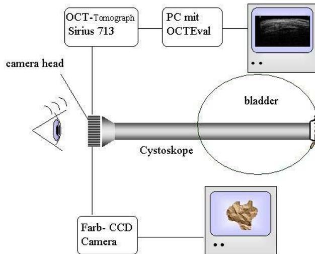
Fig. 2: Schematic overview of OCT-Cystoscopy
