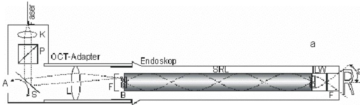
Fig. 1: OCT endoscope. The single mode fiber (LWL) is connected to the modified OCT system from the 4Optics AG. The mirror is driven by a galvanometer for a lateral scan.
